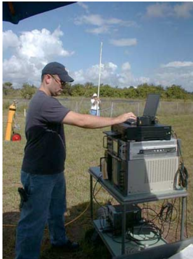
Field testing the Hydrogen fire system.
